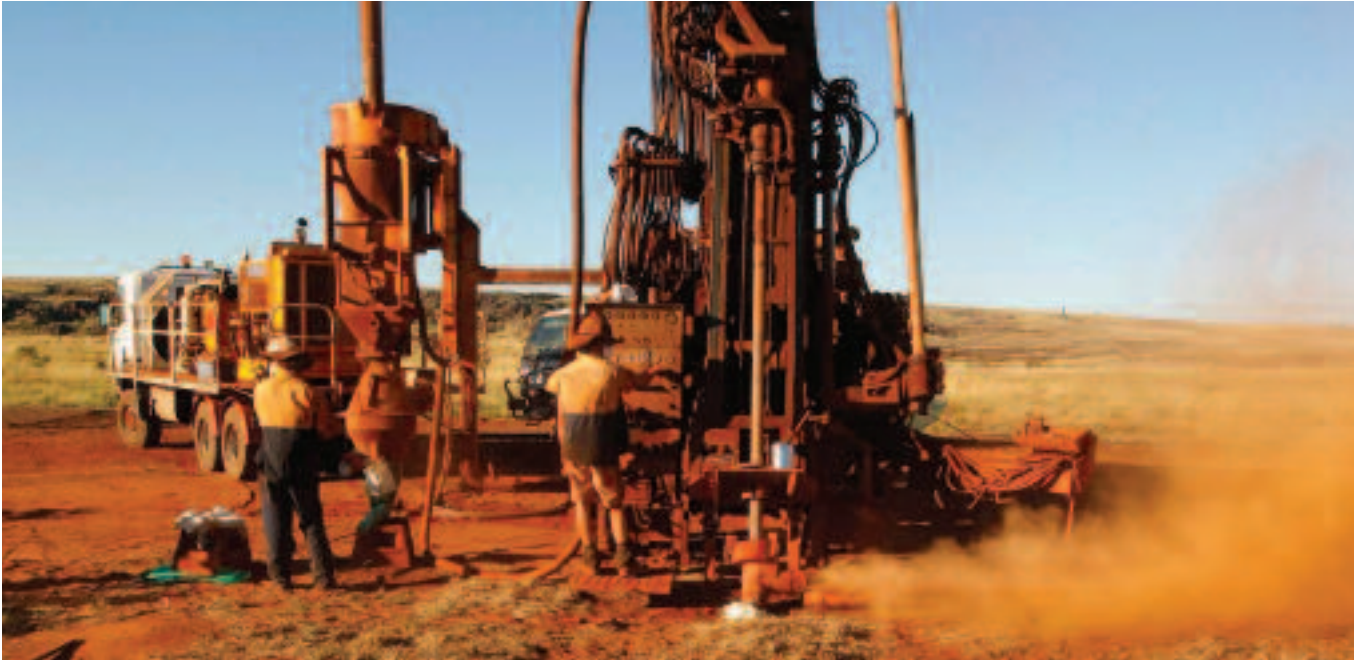
An operator controls a core drill rig at an iron ore mine site near Port Hedland, Australia.
